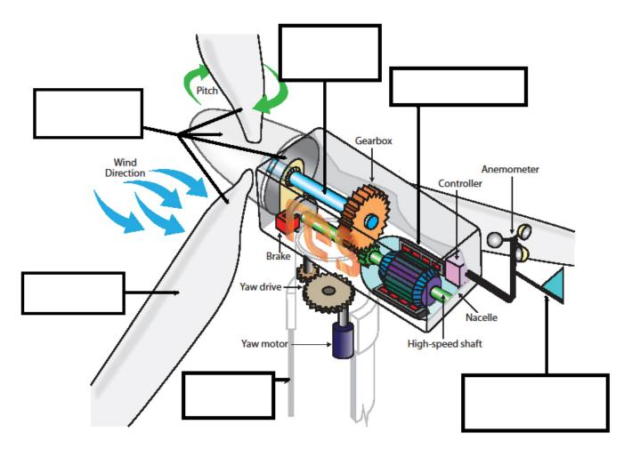
Weather vane Tower Blade Rotor Generator Low Speed Shaft
